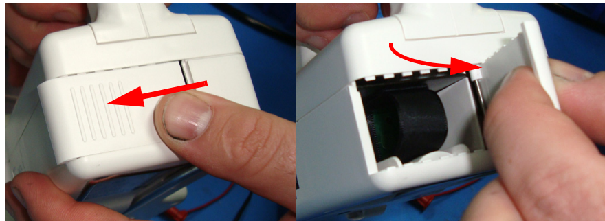
Figure 3-1 Open the battery compartment door
