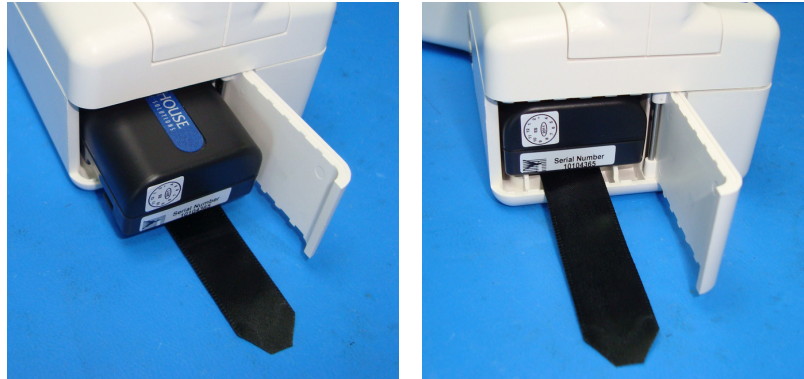
Figure 3-3 Insert battery into battery compartment
