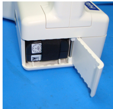
Figure 3-4 Tuck battery release ribbon
