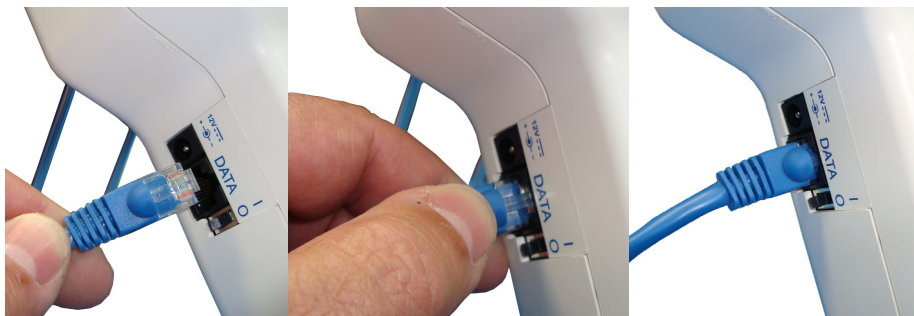
Figure 3-13 Connecting RJ-45 data communications cable
