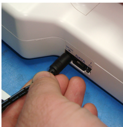
Figure 3-8 Inserting DC power plug.
