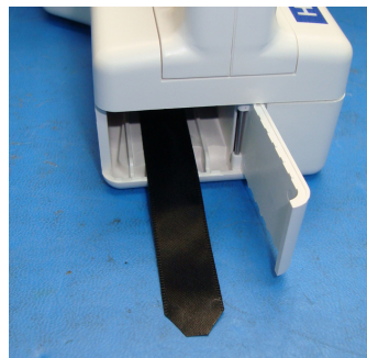
Figure 3-2 Pull Battery release ribbon out
