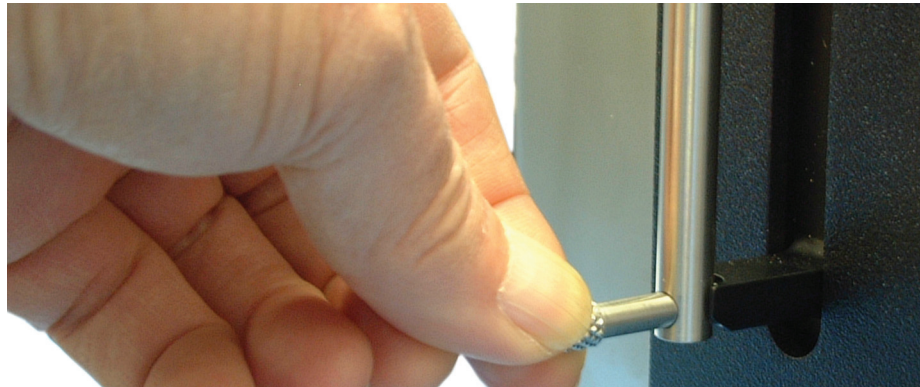
Figure 3-30 Reinstalling Plunger Rod Pin
