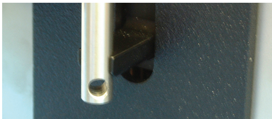
Figure 3-29 Plunger Rod and Actuator Arm Detail
