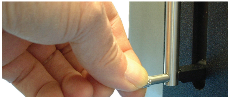
Figure 3-26 Removing Syringe Mounting Pin
